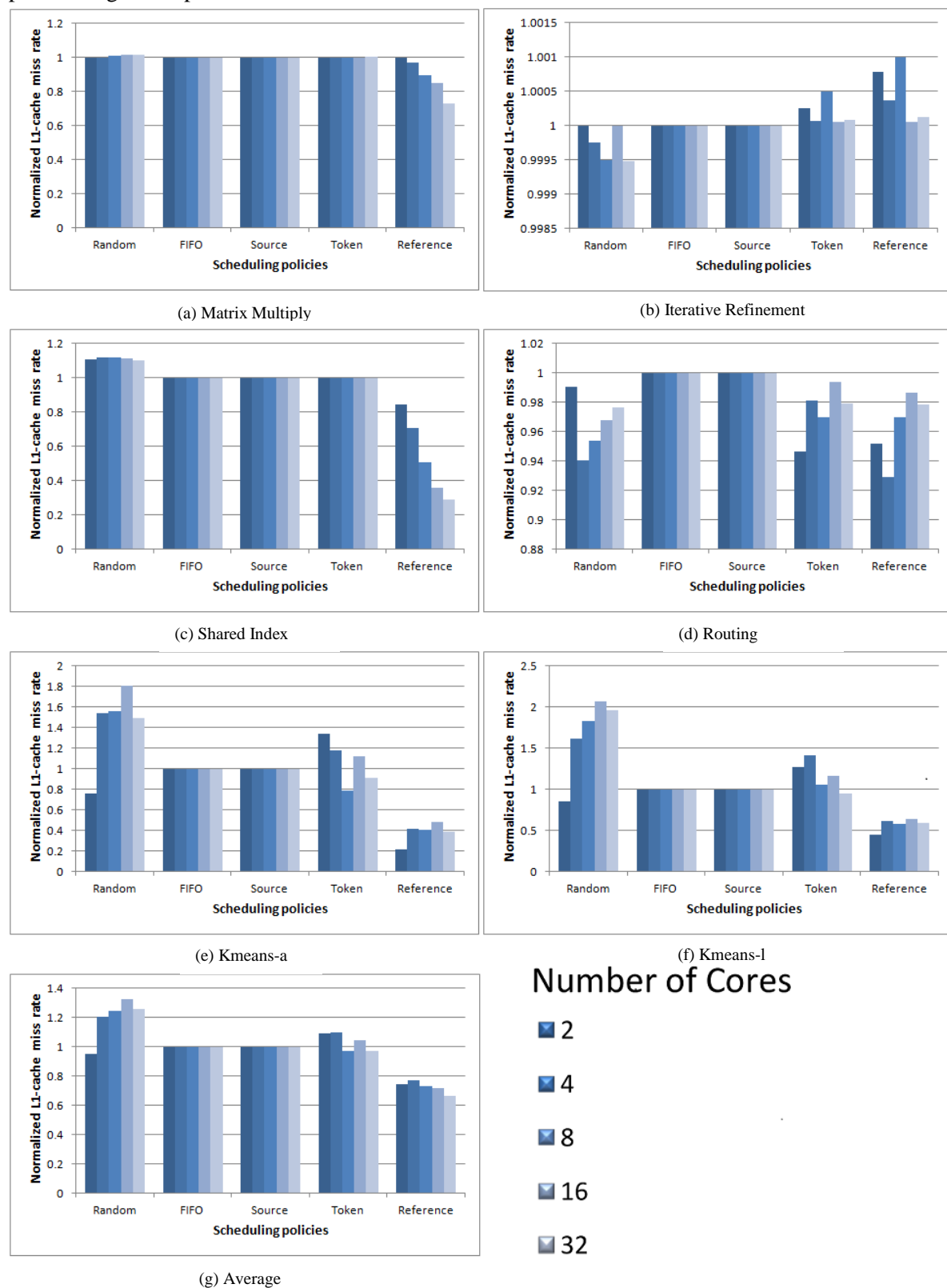
Figure 22: Number of L1 misses, as a percentage of those seen with FIFO scheduling
